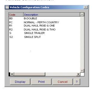
This entry screen is used to set up vehicle configurations. By entering a configuration, you are able to link the configuration along with the route code and pay type when setting up driver rates and trip rates that are used in calculating employee pays.
