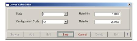
The driver rate master file entry screen is a utility used to set up driver rates. By entering a state and vehicle configuration, you are able to set a rate per kilometre or rate per hour that is used in calculating employee pays.
